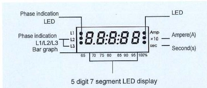
3 phase currents (In) and a leakage current (3M22/FM22) are displayed every 2 seconds in sequence.
